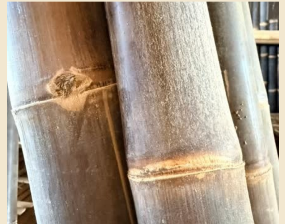
Smoked, treated structural bamboo
